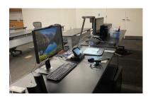
Power on the Document camera and adjust the light settings to your preference. To turn on the document camera press hold and wait for the blue light to appear. To adjust or turn on the light press the lamp button (for top & bottom lamps & off) and then use the BRIT- or BRIT+ to adjust the light.
