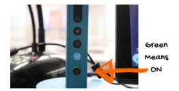
Power on the iPad/touch panel. When it is on you will see four columns (Desk Monitor; Displays 1,3,5; Displays 2,4; Projector). Each column should be set to EN-210 Room PC. Do not switch to any of the other options if you are using the room computer.
