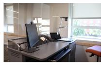
Power on the Document camera and adjust the light settings to your preference. To turn on the document camera press hold and wait for the blue light to appear. To adjust or turn on the light press the lamp button (for top & bottom lamps & off) and then use the BRIT- or BRIT+ to adjust the light.
