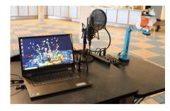
Power on the Document camera and adjust the light settings to your preference. To turn on the document camera slide the button down until you see a green semi-circle. To adjust or turn on the light press the filled in sun to dim press the empty sun.
