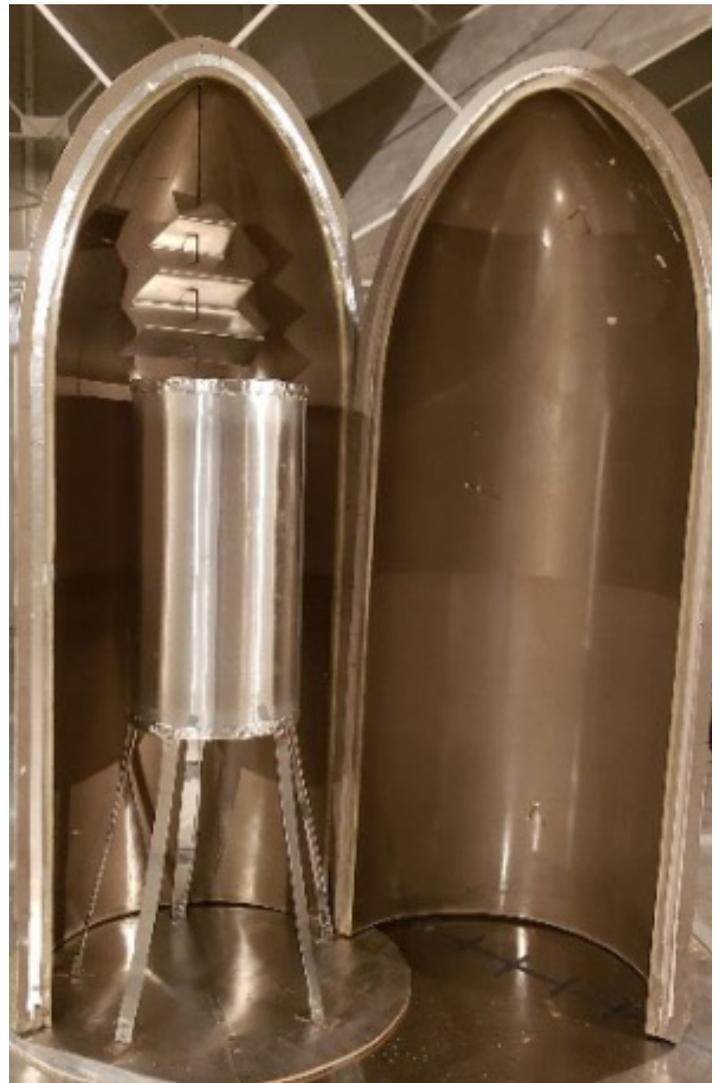
An image of a simulated payload for satellite launch.
