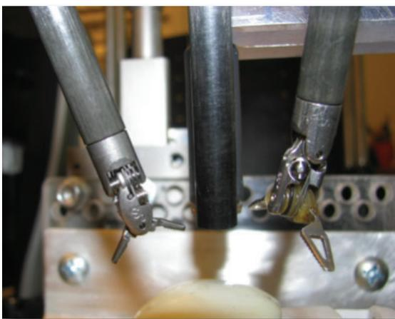
A new imaging applicator probe under development (middle) is placed alongside robotic surgical instruments
