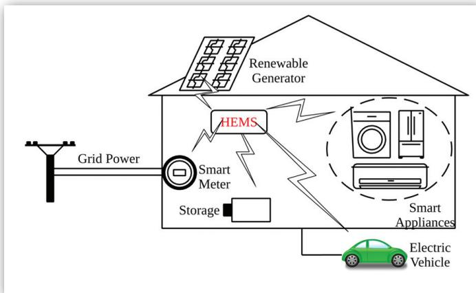
A future smart home with roof-top solar panels, electric vehicle, smart appliances and energy storage managed by the home energy management system (HEMS)
