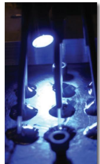
A fiber-optical array for medical research is being cured under ultraviolet light
