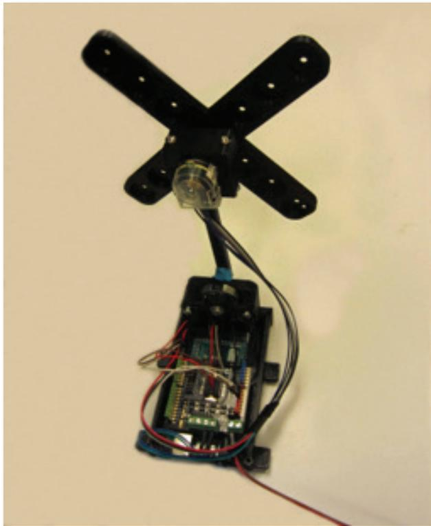
Reaction Wheel Pendulum
