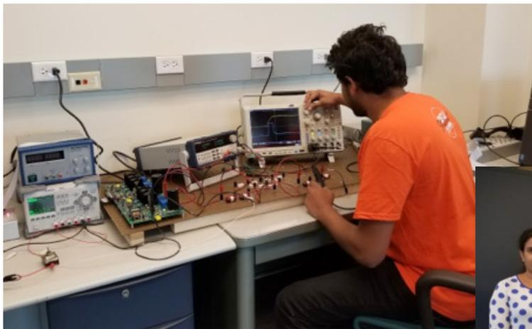
Power converter control: Graduate student Anushka Dissanayake tests a developed converter control algorithm
