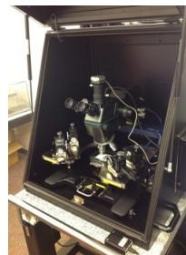
Cascade Microtech EPS150 Probe Station
