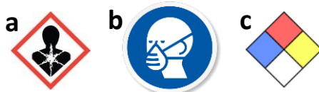
Figure 4.4.1 GHS (a), PPE (b), and NFPA Diamond (c) Signage
