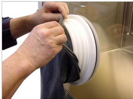
Remove both O-rings from the gloveport feedthrough
