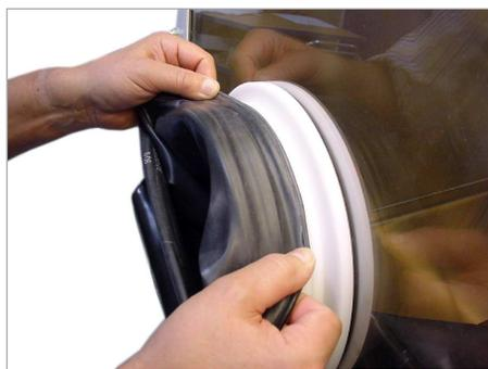
Pull old glove off the gloveport feedthrough and **IMMEDIATELY** put new glove over it.
