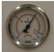
The antechamber pressure is displayed on the manometer on the antechamber. During the evacuation and refilling process:
