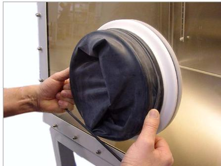
Put new glove onto the gloveport feedthrough up to the inner notch.
