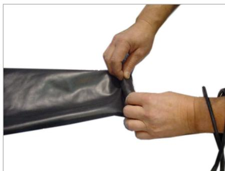
Roll new glove on firmly so that as little air as possible remains in the new glove.
