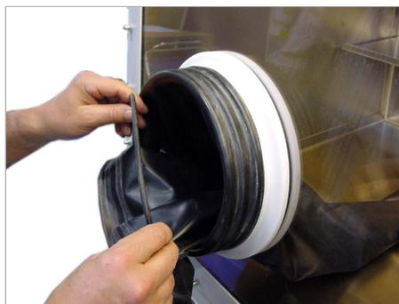
Remove both O-rings from the gloveport feedthrough.
