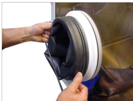
Only secure new glove first with a new O-ring on the inner notch of the gloveport feedthrough.
