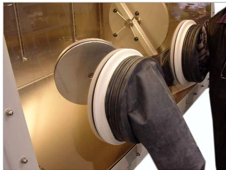
Secure glove onto the outer two notches of the gloveport feedthrough with two new O-rings.
