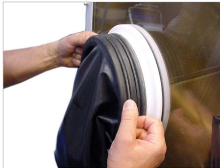
Then secure new glove with a second new O-ring on the outer notch of the gloveport feedthrough.
