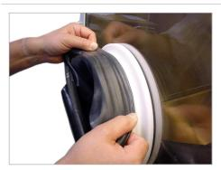
Pull old glove off the gloveport feedthrough and IMMEDIATELY put new glove over it.
