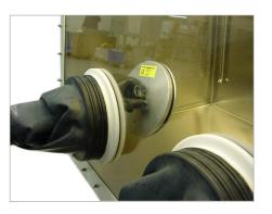
Attach inner sealing cover either through the gloveport feedthrough whose gloves should be replaced (knob is then outside) or through another gloveport feedthrough (knob is then inside).
