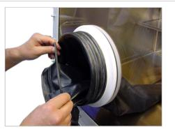
Remove both O-rings from the gloveport feedthrough.
