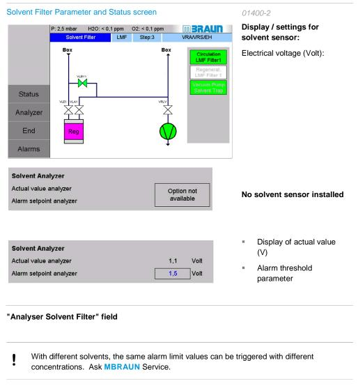
The display can be adapted to a particular solvent (optional).
