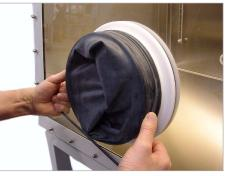
Secure glove onto the outer two notches of the gloveport feedthrough with two new O-rings. Remove inner sealing cover.
