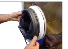
Only secure new glove first with a new O-ring on the inner notch of the gloveport feedthrough.
