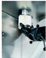
Load new filter Put on new filter and screw in
