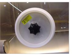
Remove both O-rings from the gloveport feedthrough Remove glove
