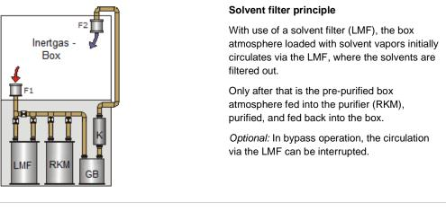
LMF Solvent filter RKM Purifier (H2O/ O2)GB Blower Heat exchanger (optional)
