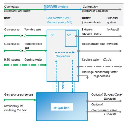
Pressure reducing valves are not part of delivery, installation is in responsibility of the customer
