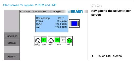
Display here: separate vacuum pump for LMF (optional)
