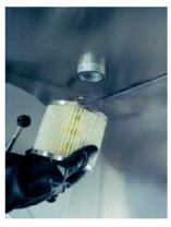
In ongoing operation: Carefully pull out used filter unit Place in a container that can be sealed Unload and dispose of properly. Carefully clean box of loose particles
