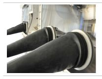
Standard boxes are equipped with round gloveport feedthroughs and butyl gloves.
