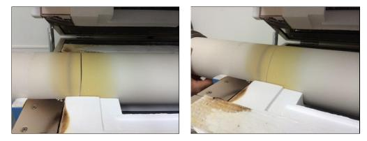
• For minimizing the possibilities of the phenomenon above, **TWO** tube blocks must be used and placed on each side of the tube at the positions depicted below:
