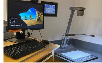
**03** Power on the Document camera and adjust the light settings to your preference. To turn on the document camera press hold and wait for the blue light to appear. To adjust or turn on the light press the lamp button (for top & bottom lamps & off) and then use the BRIT- or BRIT+ to adjust the light.
