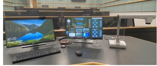
**03** Power on the Document camera and adjust the light settings to your preference. To turn on the document camera push and hold the power button. To turn on/off or adjust the light, push and hold the light buttons.
