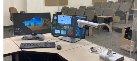
**03** Power on the Document camera and adjust the light settings to your preference. To turn on the document camera push and hold the power button. To turn on/off or adjust the light, push and hold the light buttons.
