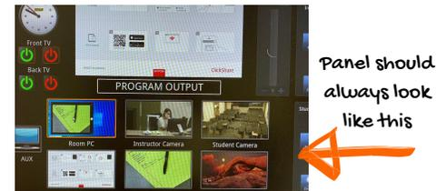
**05** Touch Panel: If the front TV is not on, select the power button on the "Front TV". There is no need to turn on the back TV unless you are streaming from Tulsa.
