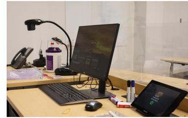
**03** Power on the Document camera and adjust the light settings to your preference. To turn on the document camera press hold and wait for the blue light to appear. To adjust or turn on the light press the lamp button (for top & bottom lamps & off) and then use the BRIT- or BRIT+ to adjust the light.
