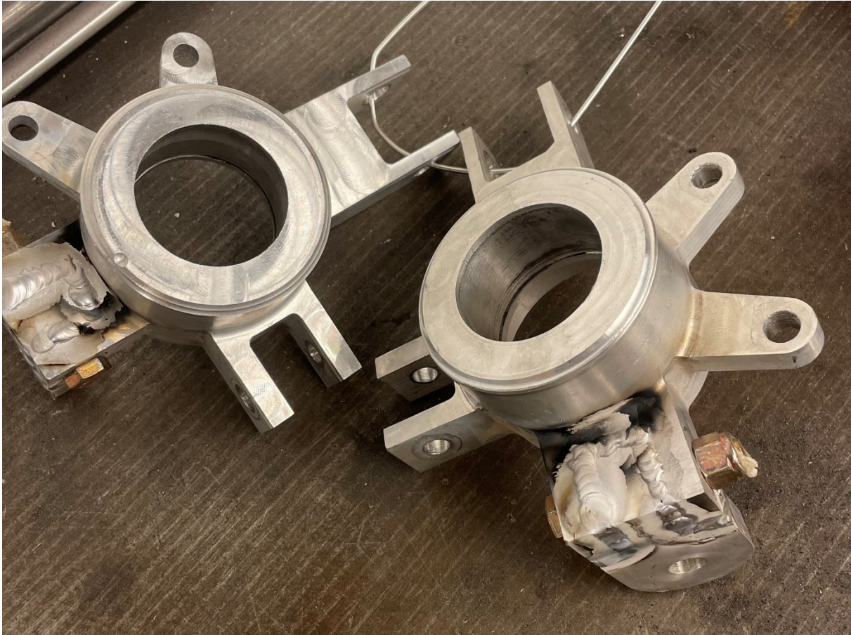
Figure 2.6: Fully Assembled Knuckle with Welded Upright
